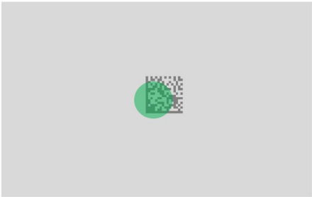
Figure 4. Relative Size and Location of Gryphon™ GFS4500's Green Spot
